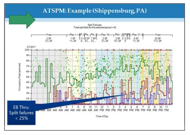
Figure 2.11 Purdue Split Fail Sequence Change Analysis (EB Thru) - PennDOT
