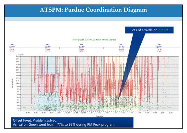
Figure 2.29 PCD Used to Identify Offset Concern (AFTER) - PennDOT
