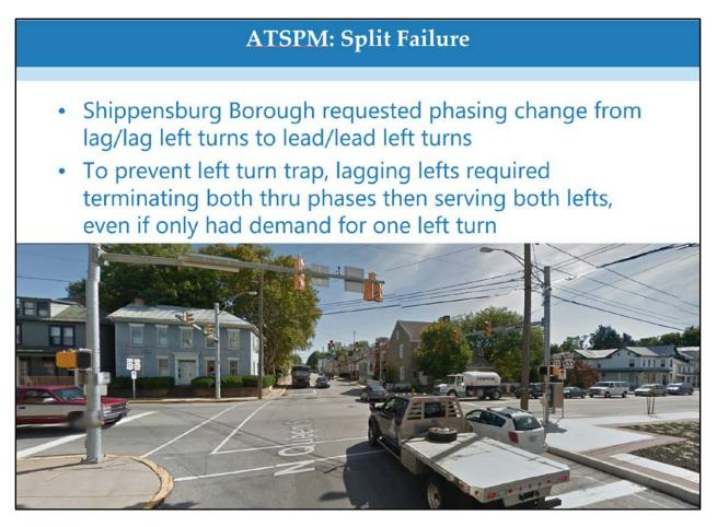
Figure 2.9 Purdue Split Fail Analysis - Sequence Change Potential – PennDOT
