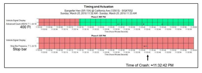
Figure 1.25 Timing and Actuation Metric – Bangerter & California - 1 minute analysis between 11:32 AM and 11:33 AM
