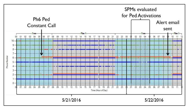
Figure 1.12 ATSPM Evaluation for High Pedestrian Activation Occurrences
