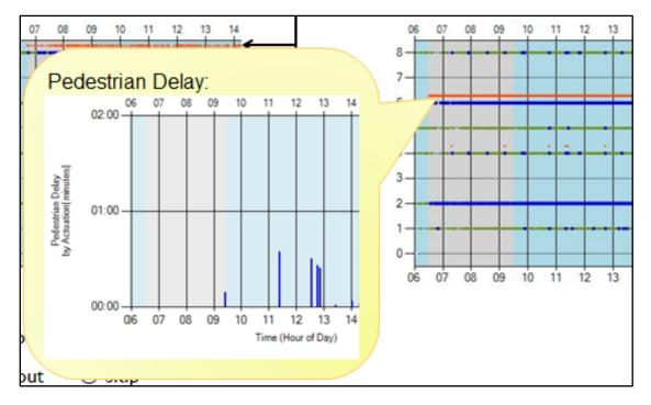
Figure 2.24 Pedestrian Delay Shows Pedestrian Actuations on Coordinated Phases
