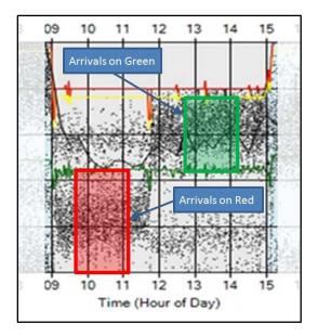
Figure 2.26 PCD Where Offset was corrected at 11:45
