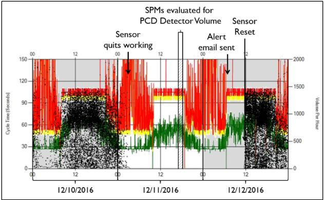
Figure 1.7 ATSPM Evaluation for Low Advance Detection Counts
