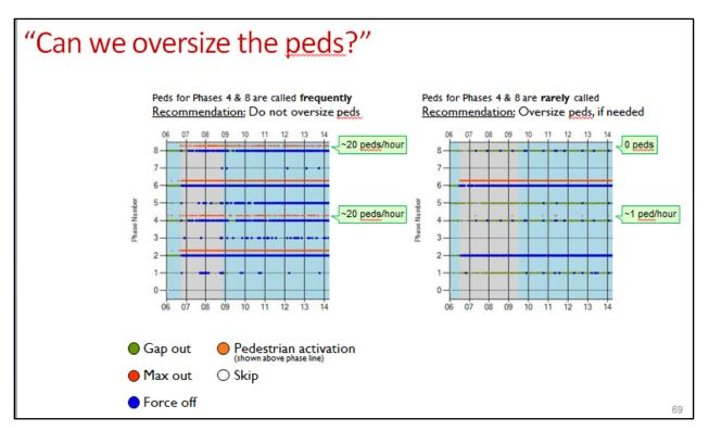
Figure 2.23 Evaluating if Pedestrian Times Can be Over-sized
