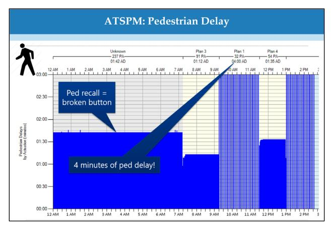
Figure 2.25 Pedestrian Delay Shows Pedestrian Actuations on Coordinated Phases - PennDOT
