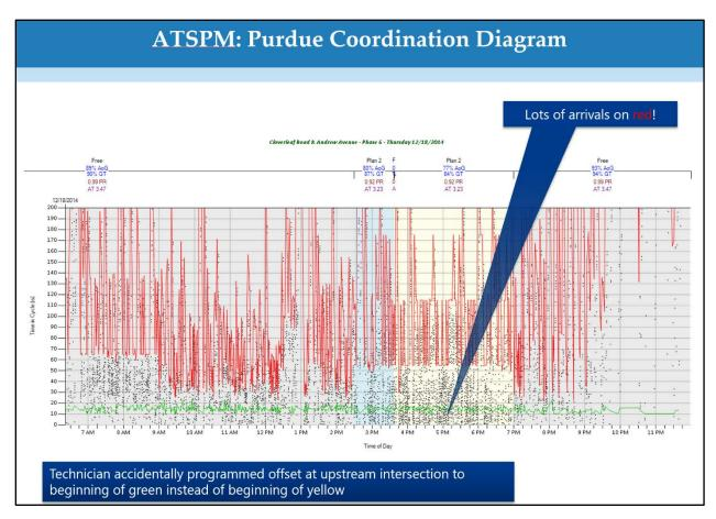
Figure 2.28 PCD Used to Identify Offset Concern (BEFORE) - PennDOT
