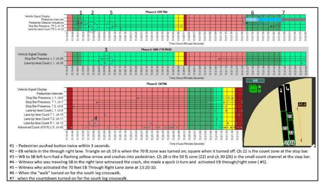
Figure 1.28 Timing and Actuation – Signal # 7510 – Time Range: 1:19:45 PM to 1:22:00 PM
