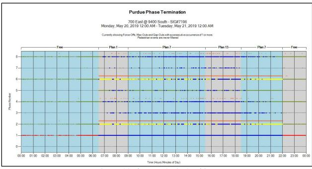
Figure 1.19 Stuck Detector Causing Complaints
