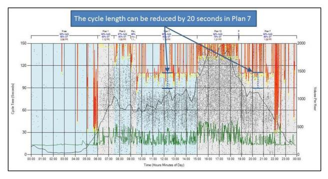
Figure 2.20 PCD Indicates Need for Lower Cycle Length - GDOT
