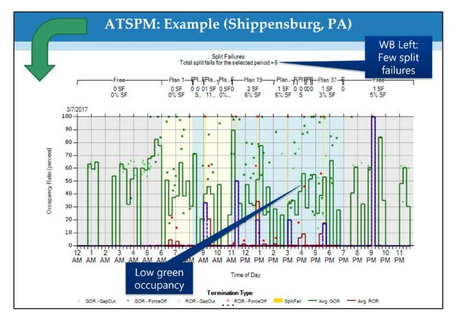
Figure 2.10 Purdue Split Fail Sequence Change Analysis (WB Left) - PennDOT
